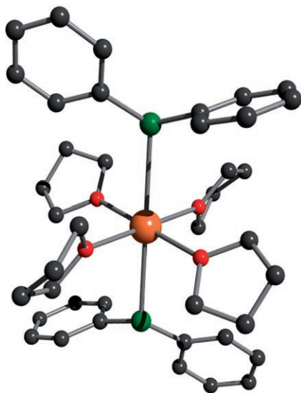
Figure 10. Molecular structure of [Ca(PPh 2 ) 2 (thf) 4 ] (color code see Figure 1, P green). Hydrogen atoms are omitted for clarity reasons.
